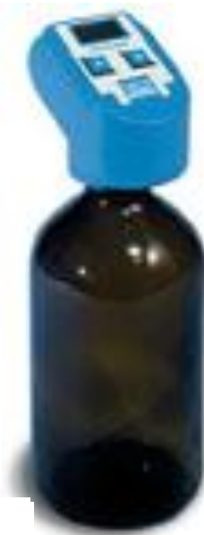
Bottle equipped with pressure-measuring head
